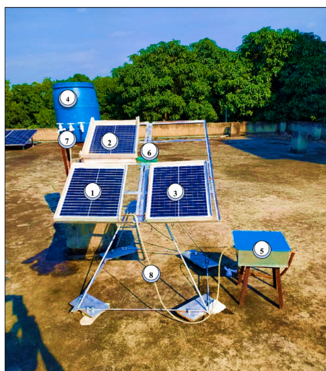
Fig. 2. Experimental setup of PVT hybrid nano-PCM (PVT/HNPCM) system.
